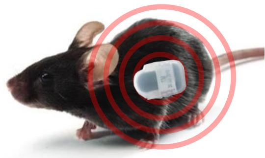
Implantable radiotelemetric transmitters enable the continuous collection of physiological data, e.g. pressure or biopotential signals, respiration rate, body temperature or activity, in conscious freely moving animals.
