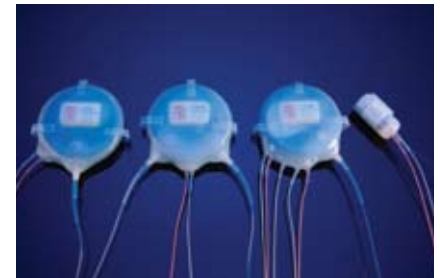
Transmitters are provided in packages of various sizes in order to optimize features, battery life, and transmitting range.
